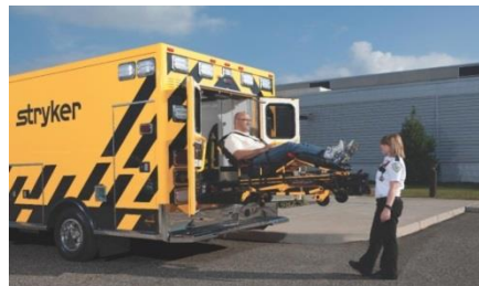
Figure 8-5: Bariatric Ambulance Power Load Systems
